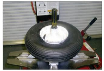
**B202.** Position the Snake<sup>™</sup> tool and remove the top bead. Next remove the second bead.
