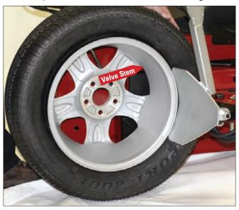
Figure 23 - Loosen Bottom Bead
