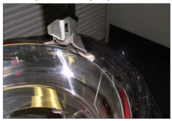
Next, jog the machine rotation a short distance and observe the bead removal. Continue to rotate the rim until the bead is completely removed.
