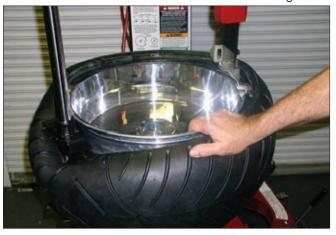
**207.** Use the RoboArm to push down on tire and swing duckhead from rim position.
