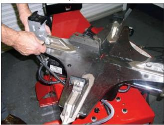
**103.** As with motorcycle clamps, after bead loosening and before clamping the wheel, preposition the clamps.
