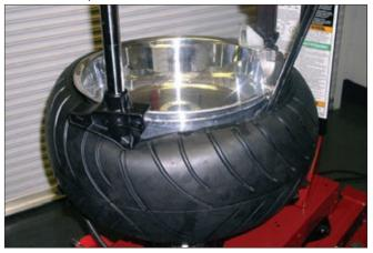
**109.** If may be necessary to push the tire sidewall down at several locations to ease the stress in the tire bead.
