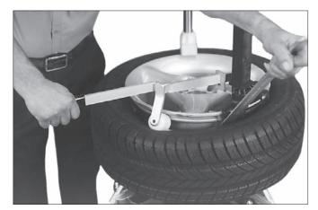
Figure 28 - Insert Bead Lifting Tool
