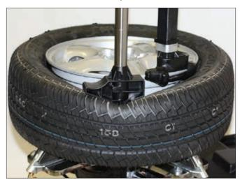
Figure 25 - Helper Foot Depressing Sidewall of Tire
