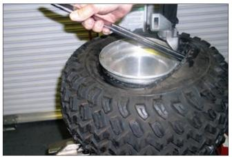
**A204.** To remove the lower bead on very wide tires, the lever bar may be placed under the lower bead and rotated up.
