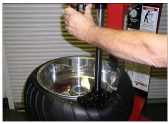
**106.** Lubricate the upper bead surface. To assist, position the manual roller assembly into the receiver. Press down and the roller between the rim and the tire bead. This will allow easy lubrication of the upper bead surface and rim flange.
