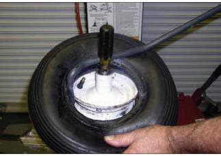
**B206.** A pair of regular vice-grip type pliers attached to the rim may be used to hold the bead lock.
