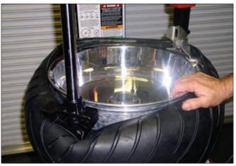
**206.** Reposition the RoboArm back to 90-degrees forward of the duckhead and finish the mounting.
