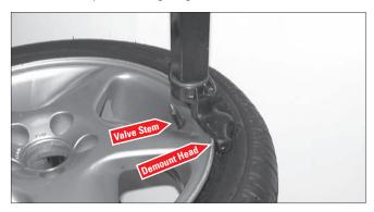
Figure 27 - Position Valve Stem Under Demount Head
