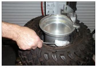
**A203.** Using typical procedures, remove upper bead.
