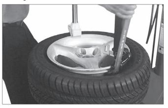
Figure 29 - Rotate Lifting Tool Down for Demount
