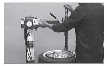
Figure 7 - Adjust Swing Arm to Position Tool Roller
