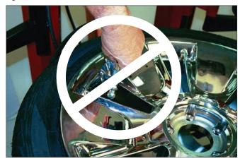
Figure 19 - Do Not Use a Hand-held Style Air Chuck
