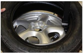
Figure 14a - Position Tire Against Mount/Demount Tool
