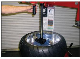
**105.** To assist in positioning the duckhead at the location near the rim, use the Robo Arm to press the tire sidewall down.
