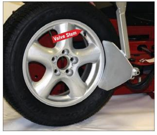
Figure 20 - Position Tire for Bead Loosening
