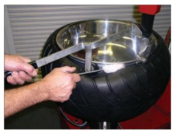
107. Insert the smooth curved end of the bead lifting tool over the forward end of the demount tool and below the top bead of the tire. Lift the bead up and over the knob on the demount tool. Also, note the valve stem position to the demount tool. Use the Robo-Arm® to push down on the tire opposite the demount tool to allow the bead to utilize the drop center area of the rim, this position reduces stresses in the bead and allows an easier bead lift.
