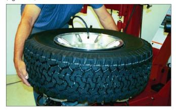
Figure 16 - Lift Tire Upwards for Bead Sealing
