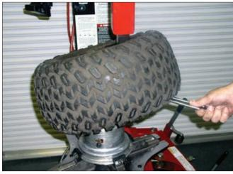
Mounting ATV Type Wheels/Tires Down To 8-inch Diameter
