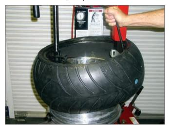
**111.** Lower bead removal is typical with standard procedures. The RoboArm may be used to assist in holding the lower bead up in the wheel's drop center.
