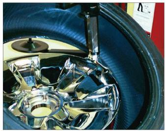
Figure 31 - Mount the Lower Bead
