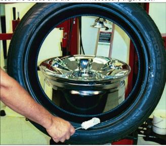
Figure 30 - Lubricate Tire Beads
