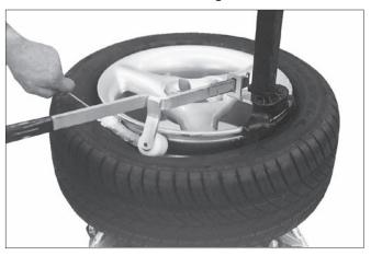
Figure 26 - Lubricate Upper Bead
