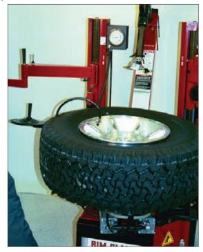
Figure 17 - Stand Back during Bead Seat
