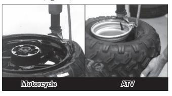
Figure 9 - Insert Bead Lifting Tool
