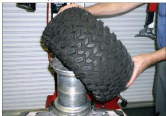
**A206.** Top bead is mounted using typical procedures.
