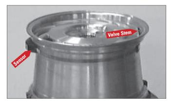
Figure 22 - Wheel with Low Pressure Sensor/Transmitter
