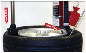
Figure 8a - Insert Bead Lifting Tool
