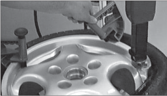
Figure 27 - Remove Drop Center Tools
