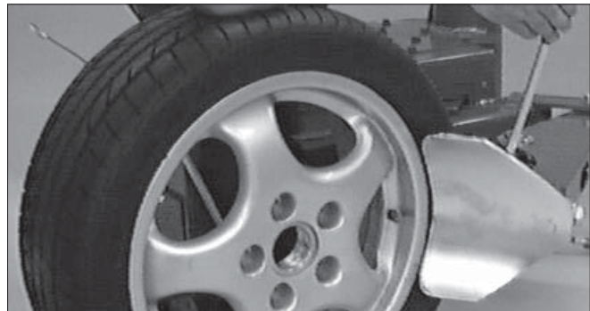
Figure 18 - Position Tire for Bead Loosening
