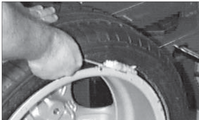
Figure 22 - Lubricate Bottom Bead
