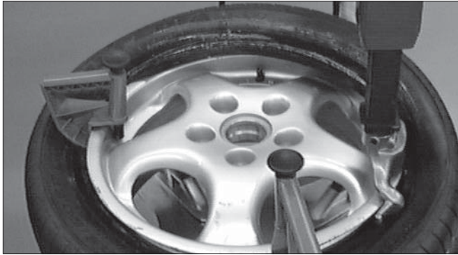
Figure 31 - Add Second Drop Center Tool
