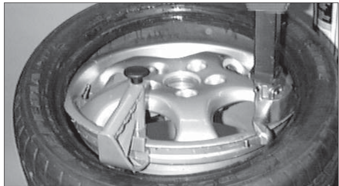
Figure 30 - Mount Top Bead
