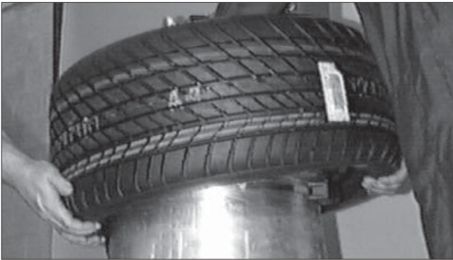
Figure 28 - Use Help on Lower Bead, Watch Sensor
