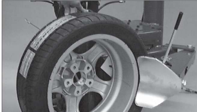
Figure 21 - Loosen Bottom Bead
