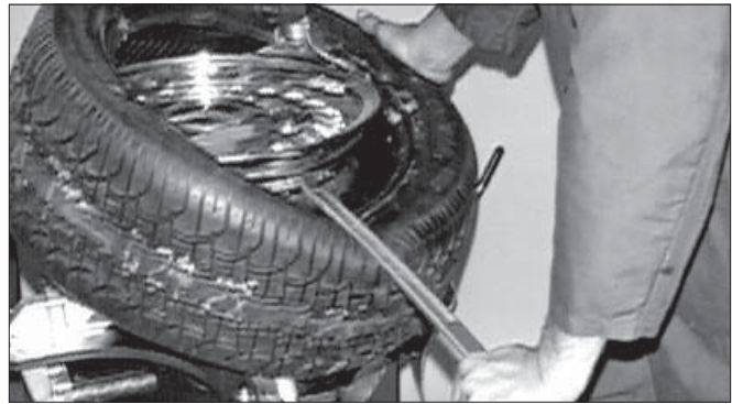
Figure 29 - Mount Lower Bead, Use Lifting Tool
