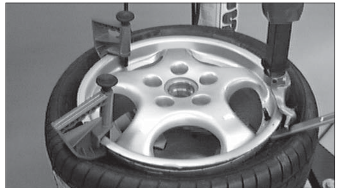
Figure 25 - Insert Bead Lifting Tool (Optional Drop Center Tools Shown)
