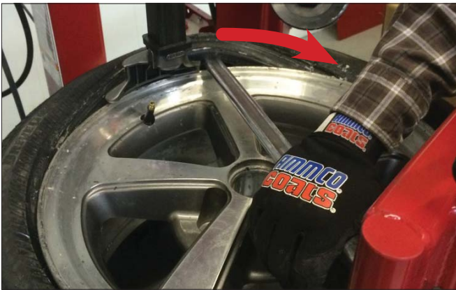
Figure 12 - Demount Upper Bead
