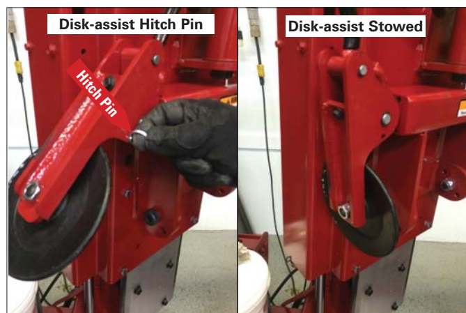
Figure 15 - Stow the Disk-assist Away
