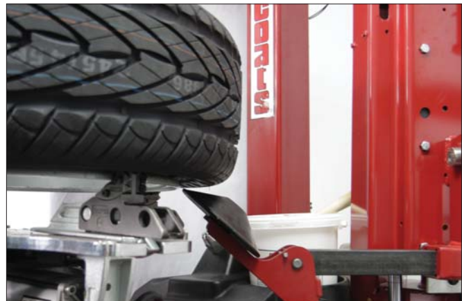
Figure 14 - Disk-assist Aiding Lower Bead Demount
