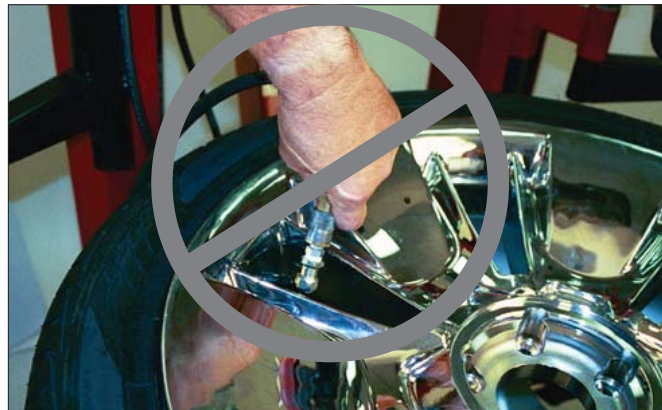
Figure 27 - Do Not Use a Hand-held Style Air Chuck
