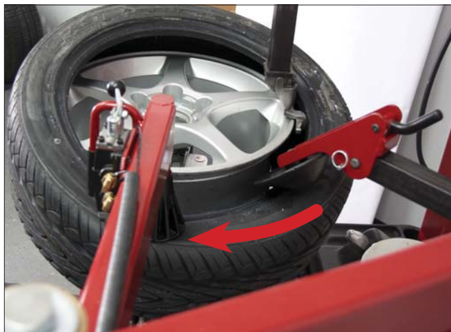
Fig 21 - Hold Tire Bead In Rim Drop Center
