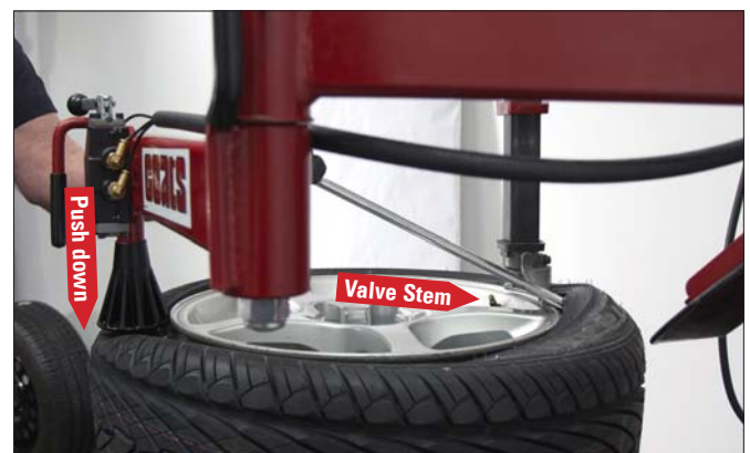
Figure 11 - Insert Bead Lifting Tool
