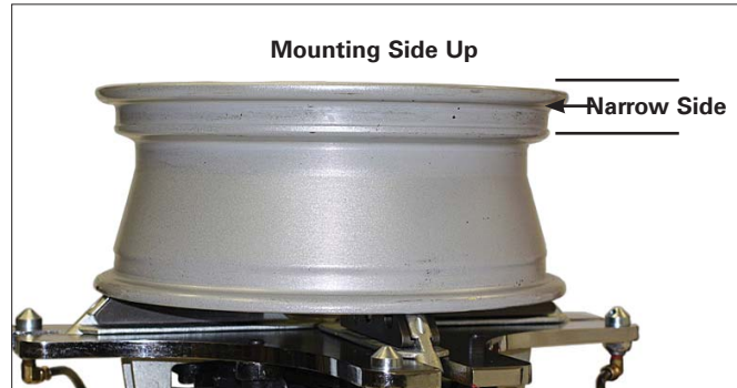
Figure 6 - Place Tire/Wheel Assembly on Table top
