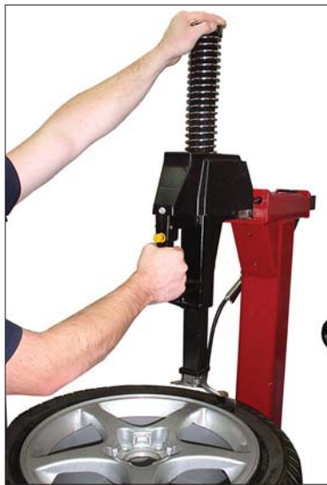
Figure 9 - Position Mount/Demount Tool
