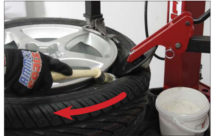
Figure 10 - Apply Rubber Lubricant to the Beads
