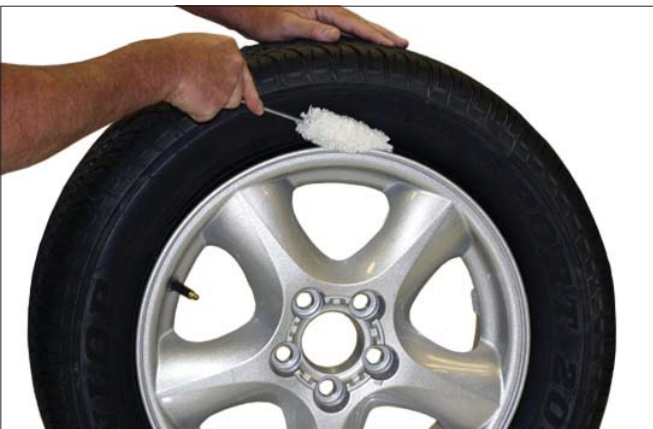
Figure 5 - Apply Rubber Lubricant to Tire Beads
