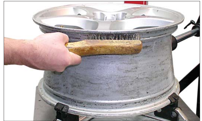
Figure 17 - Inspect and Clean the Wheel
