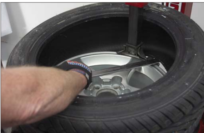
Figure 13 - Guide Lower Bead Over Knob On Demount Tool
