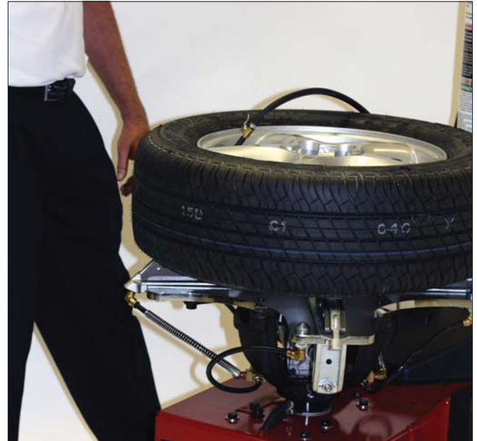
Figure 25 - Stand Back during Bead Seat
