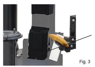
After having positioned the machine, in its final location, remove the accidental tilting safety pin from the arm (fig. 3).
