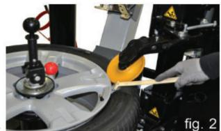
As soon as enough space is available, a proper tire lubricating paste should be carefully applied to both the inner surface of the rim and the tire bead (fig. 2).
