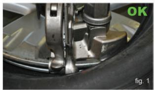
Bead correctly positioned over the left side of the mounting tool and under it on its right side.
