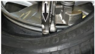
Bead correctly positioned over the left side of the mounting tool and under it on its right side, thus it can be slightly lowered for easy tire mounting.
