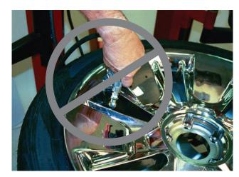
Figure 28 - Do Not Use a Hand-held Style Air Chuck
