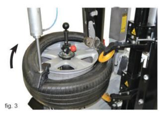
Press the pedal **2** to rotate the wheel clockwise, contemporarily press the tire manually from **"5 o'clock"** position to force the upper bead at drop-centre position. Keep it pressed while rotating up to **"8 o'clock"** position to complete the upper bead mounting (fig. 2).
