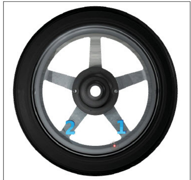
Figure - Spoke 1 and Spoke 2 Locations On Either Side Of Original Outboard Weight Location
