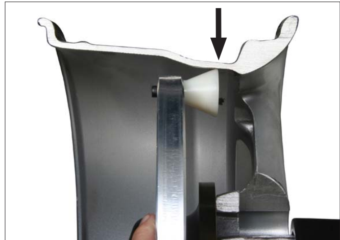
Figure 7A - Hidden Weight Location Viewed on a Cut-Away Rim for Clarification.
