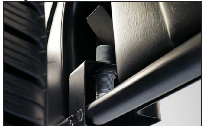
Figure 10 - Tire Width Sonar Located Inside Hood
