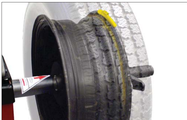
Figure 20 - Calibration Weight On Outside Flange At Top-Dead-Center
