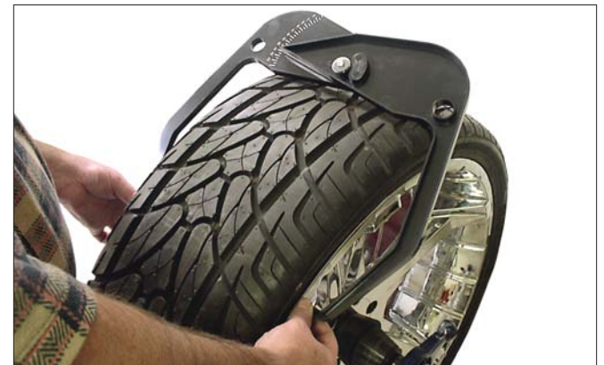
Figure 13 - Caliper Placement On Wheel
