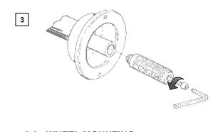
The wheel balancer is supplied complete with cone type adapter for fastening wheels with central bore. The threaded terminal is fitted according to the drawing; it can be removed to fit optional adapters.
