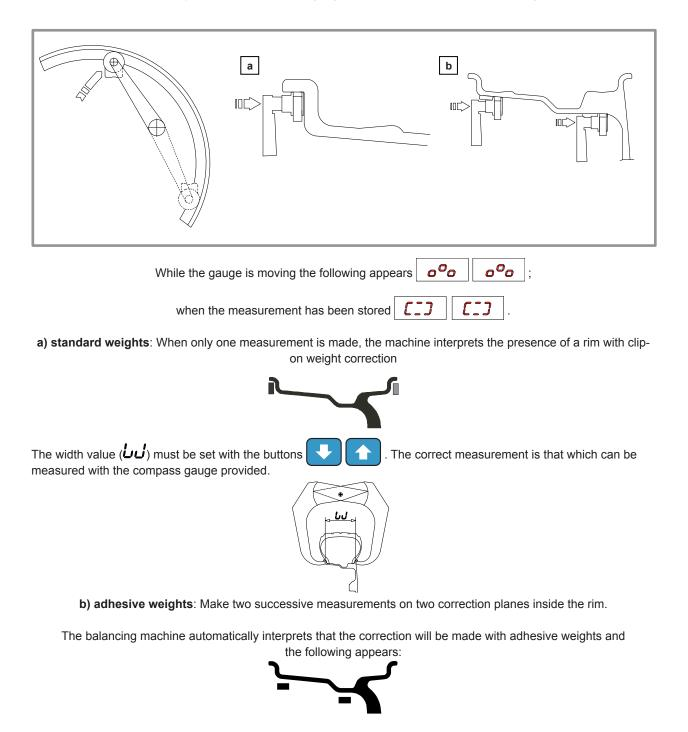
For a different combination of the type or position of the weights on the rim, use the button
