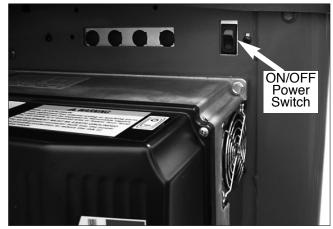
Figure 4 - On/Off Switch
