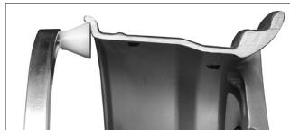
*Figure 1 - Clip-On Weight Location* Note the value entry of A & D dimension.
