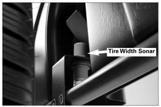
Figure 10 - Tire Width Sonar Located Inside Hood
