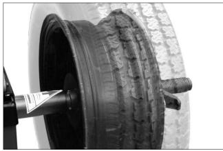
Figure 20 - Calibration Weight On Outside Flange At Top-Dead-Center
