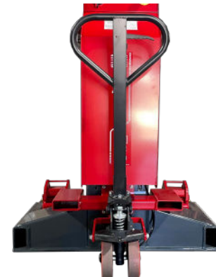
STEERING HANDLE WITH LOWERING & LOCKING CONTROL
