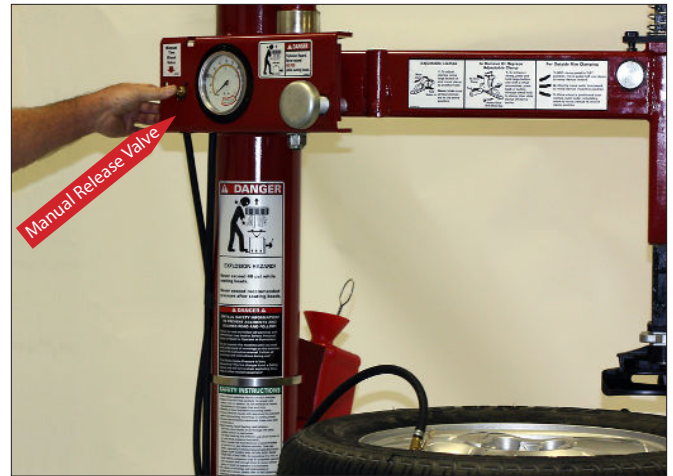
Figure 27 - Location of Manual Release Valve
