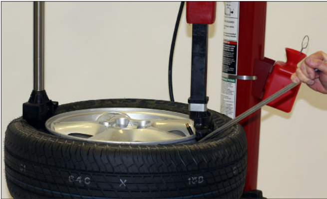
Figure 38 - Helper Foot Pushing Bead Into Drop Center
