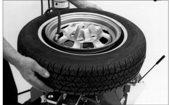
Figure 25 - Lift Tire Upwards for Bead Sealing
