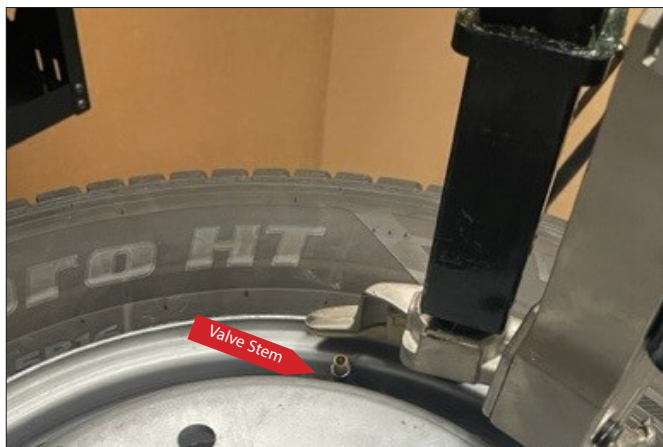
Figure 50 - Position Valve Stem Behind Leverless Demount Tool
