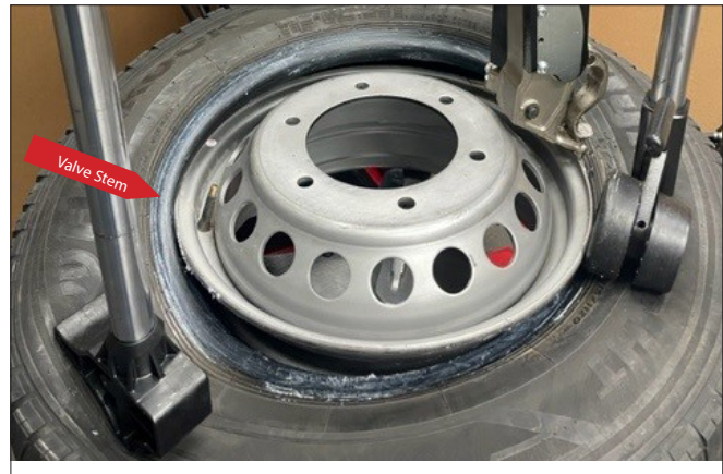
Figure 60 - Robo-Arm and Robo-Roller Pushing Tire Bead in to the Drop Center
