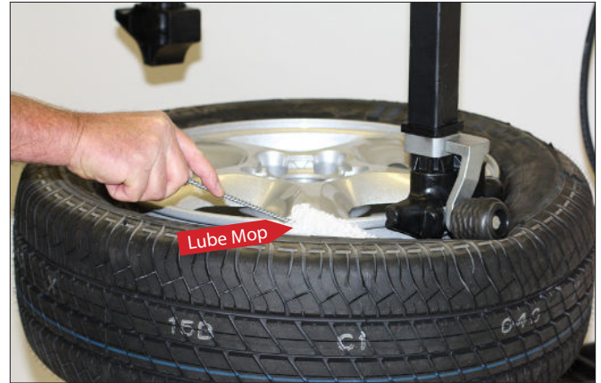
Figure 35 - Lubricate Upper Bead
