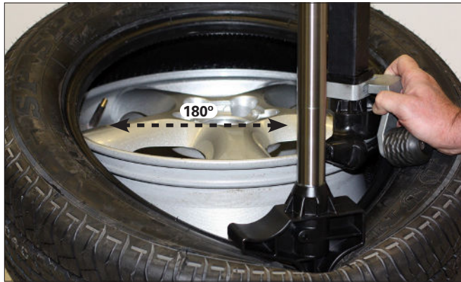
Figure 43 - Position Valve Stem 180° Ahead of Mount/Demount Tool
