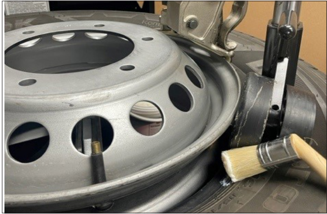
Figure 49 - Apply lubricant with Robo-Roller.
