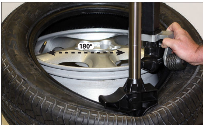
Figure 21 - Position Valve Stem 180° Ahead of Mount Tool
