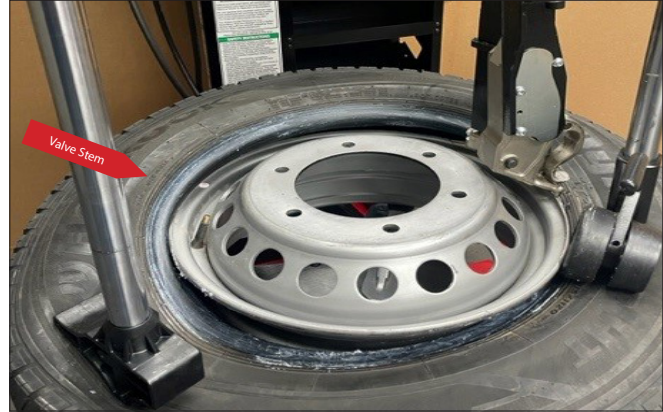
Figure 59 - Position Valve Stem In Front Of Bead Lock
