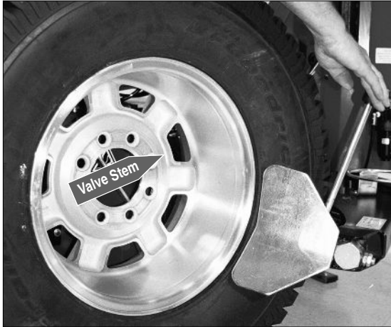
Figure 28 - Loosen Bottom Bead
