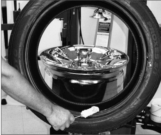
Figure 38 - Lubricate Tire Beads
