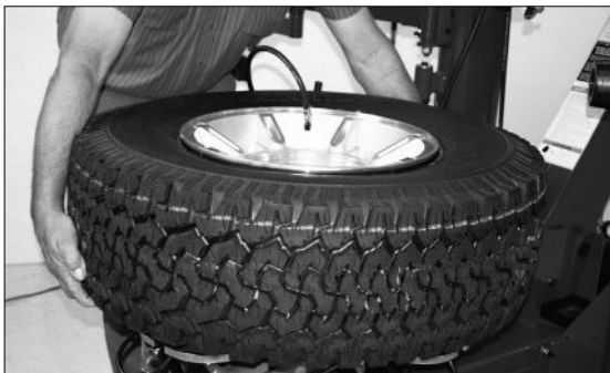
Figure 20 - Lift Tire Upwards for Bead Sealing
