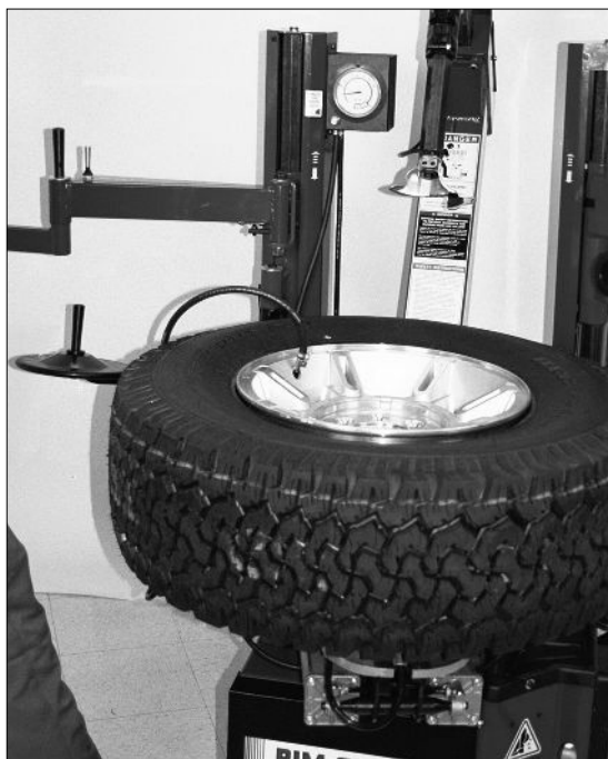
Figure 21 - Stand Back during Bead Seat
