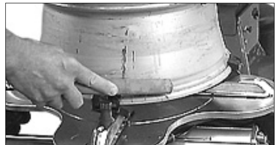
Figure 15 - Inspect and Clean the Wheel
