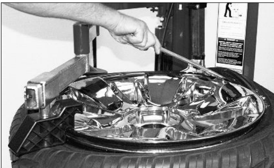
Figure 34 - Lift Bead Carefully onto Duckhead
