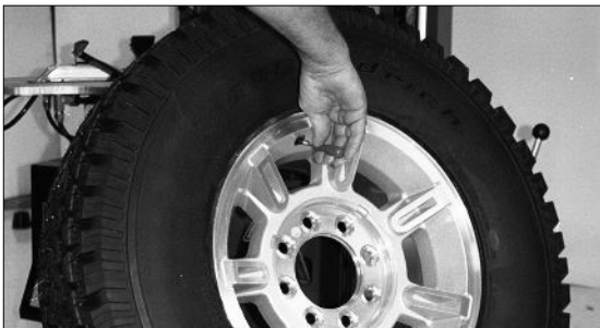
Figure 1 - Remove Valve Core to Deflate Tire
