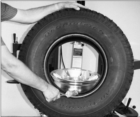
Figure 16 - Lubricate Tire Beads Liberally
