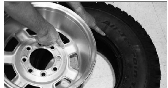
Figure 14 - Verify Size Match Between Tire and Wheel
