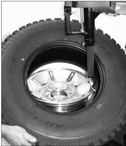
Figure 17 - Position Tire Against Duckhead
