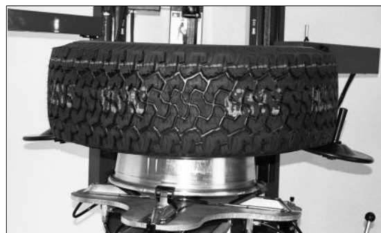
Figure 12 - Lift the Tire for Lower Bead Removal
