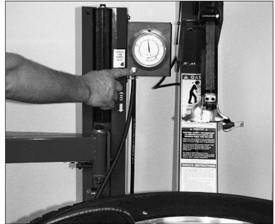
Figure 22 - Location of Manual Release Valve
