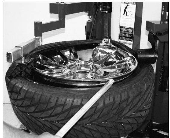
Figure 42 - Utilize the Lift Tool if Necessary
