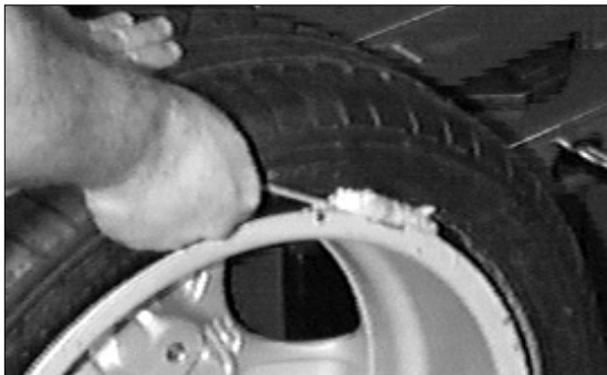
Figure 29 - Lubricate Bottom Bead
