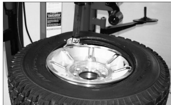
Figure 11 - Demount Upper Bead
