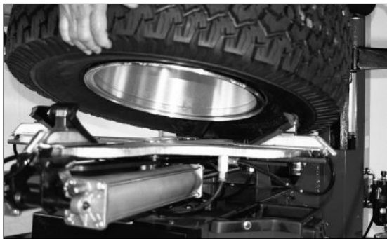
Figure 5 - Clamp Outside on Mag Wheels
