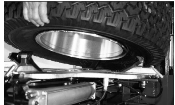
Figure 31B - Outside Clamped with Tire Removed
