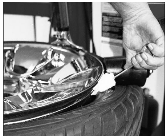
Figure 32 - Lubricate Upper Bead
