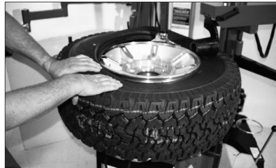
Figure 19 - Mounting Top Bead
