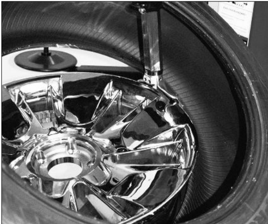
Figure 39 - Mount the Lower Bead
