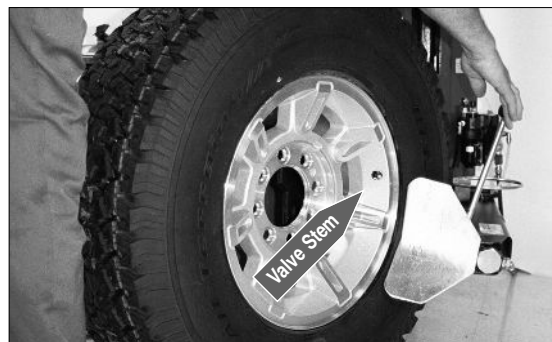
Figure 3 - Position Tire and Bead Loosener Shoe
