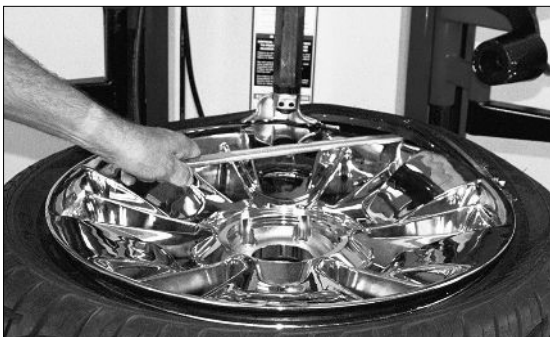
Figure 35 - Start Upper Bead Removal
