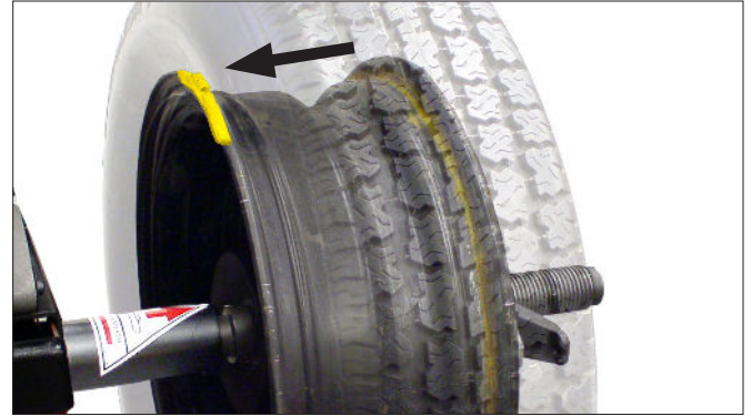
Figure 25 - Calibration Weight On Inboard Flange At Top-Dead-Center
