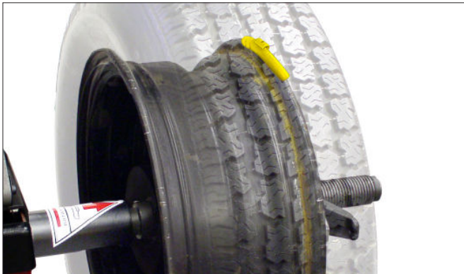
Figure 24 - Calibration Weight On Outboard Flange At Top-Dead-Center
