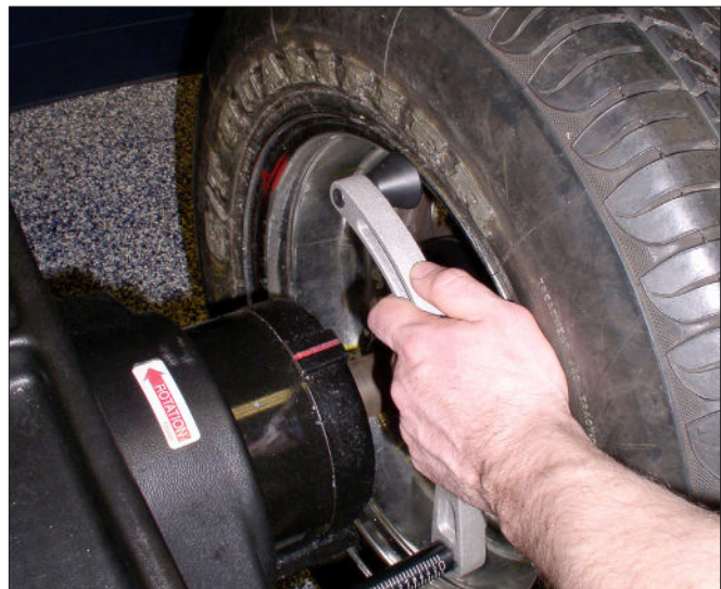
Figure 7- Automatic A & D Measurement At Clip-on Weight Location
